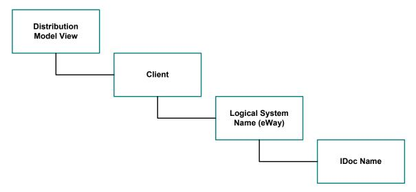
Following this high-level setup, you need to define Communications parameters in SAP R/3 to specify the correct routing of IDocs (either inbound to or outbound from SAP R/3). The hierarchy of this Communication system is shown in Figure 22. The individual steps involved in the configuration are:
